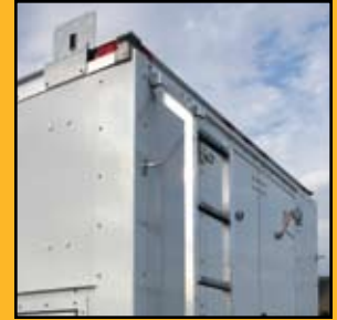
Rear Mounted Ladder (For Accessing Roof Mounted Racks)
